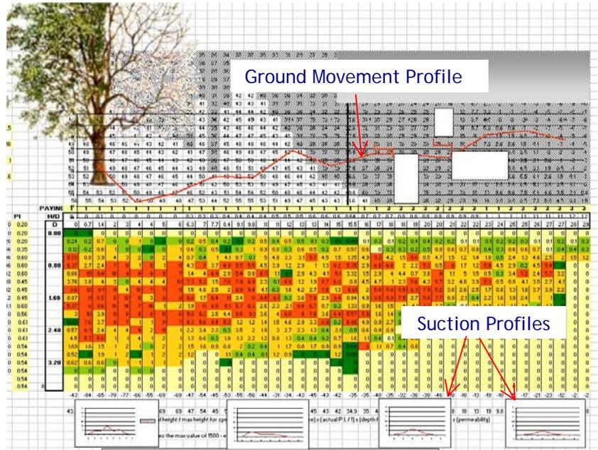
The model estimates ground movement of between 70mm close to the tree, reducing to less than 20mm or so at its 'root influence zone' periphery and below we have extracted the ground movement profile from the image above to clarify this.
