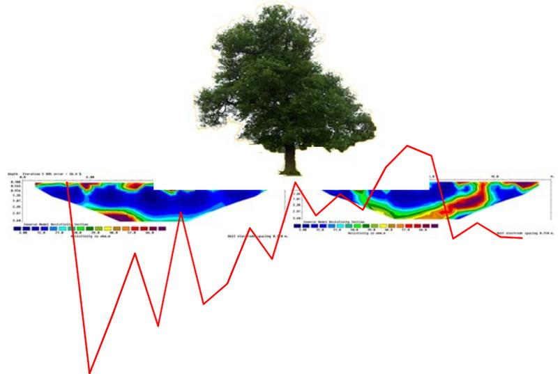
Station 21 has always been a 'high spot', moving less than its neighbours and we see in the ERT values the dark blue associated with rehydration in this location, and immediately to the right of this, at Station 22 and 23, the oranges and reds associated with dry soil where the levels confirm greater subsidence and slower recovery. Maximum movement recorded was 34.8mm at Station 9.
