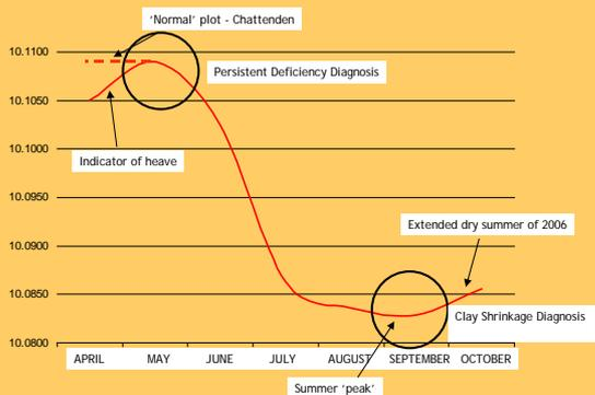
The web based interpretation application identifies root induced clay shrinkage by identifying small amounts of movement over short periods of time and uses the data 'in the alternative' - where we don't see this pattern, then clearly it will be something other than seasonal movement.
