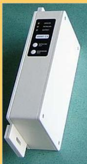
The new style sensors are much smaller units, housing the battery, electrolevel and wireless technology in a small, self-contained unit.
