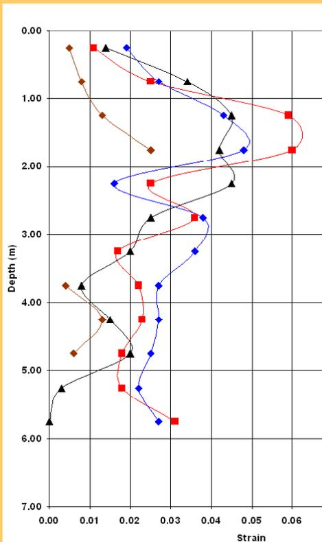
The estimate of heave was 76mm using the filter paper method and about 80mm using the oedometer. Estimates of heave are often conservative, and the modelled value of 50 - 70mm is probably more realistic.
