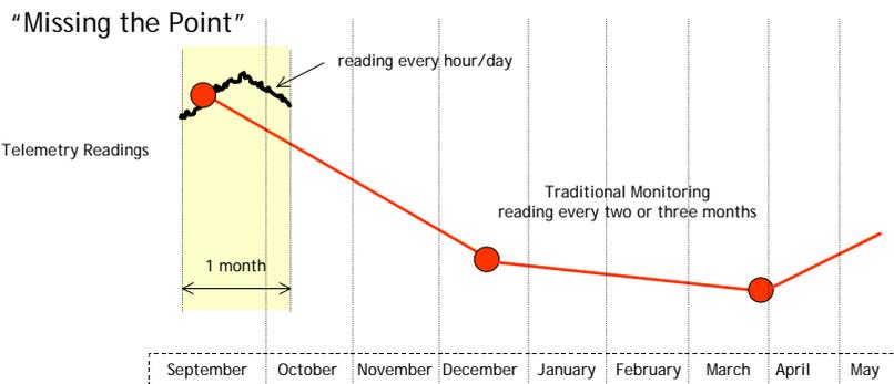
From the commercial point of view, the technology is cheap and reliable, saving both time and unnecessary disruption.
