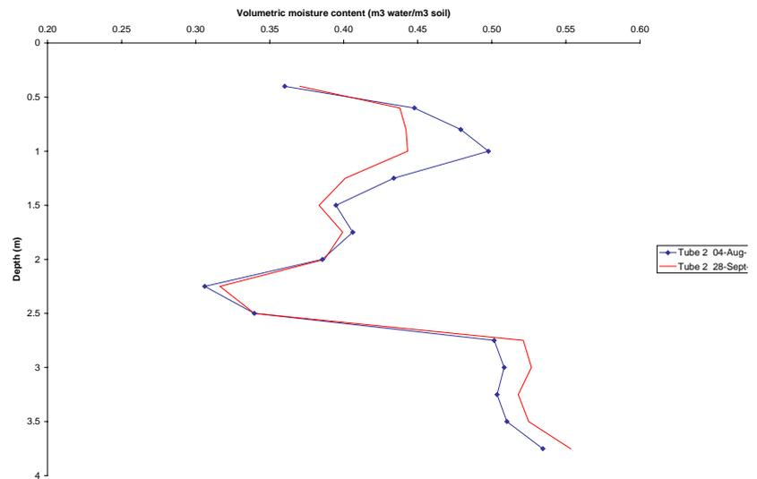
Below is the readout from the TDR and temperature sensors, received via the web. We can see the unit was live on the 24<sup>th</sup> September 2006, and the first reading was taken at 21.47 hours.
