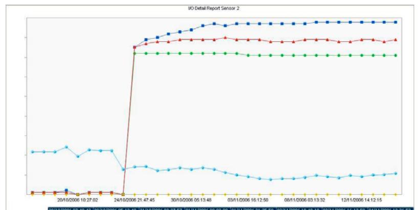
The temperature dropped from a starting point of 13.75 degrees in the office environment, to less than 8 degrees or so on site and the moisture content of the ground is rising steadily from 41% to 43.5% expressed volumetrically.
