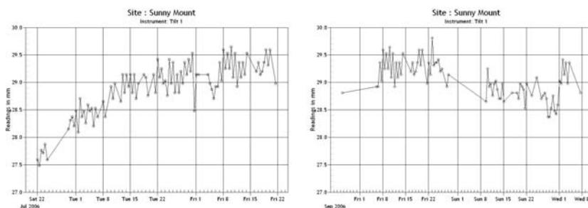
The technology has proven to be robust, transmitting information with very few lapses, recording the crucial point of contraflexure and allowing diagnosis to be made much quicker than might otherwise be the case.
